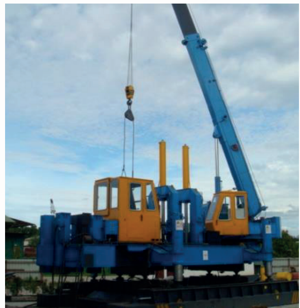
240 Tonne Injection Piling Rig
