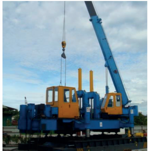
240 Tonne Injection Piling Rig
