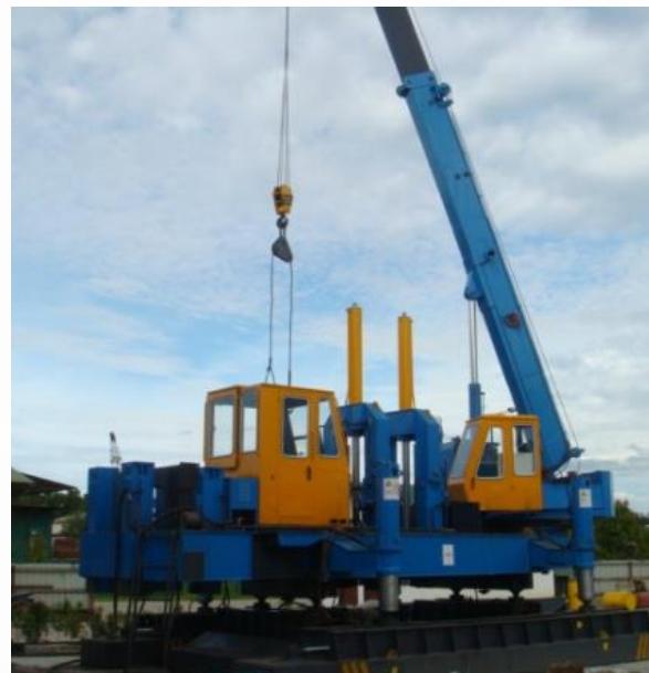
240 Tonne Injection Piling Rig
